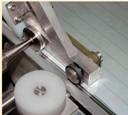
*Fig. 1 — The ultrasonic welding process attaches aluminum conductors to treated glass so that interconnects between photovoltaic cells can create an array with sufficient voltage and current to provide a practical source of electrical power.*
