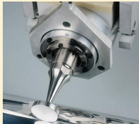
*Fig. 2 — For manufacturers of solar cells, as well as aluminum and copper foil processors, ultrasonic welding offers the fastest and highest quality method of welding.*
